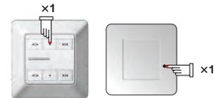
2)Short press the stop button of A channel, and then short press learning button of the emitter once, you can control the motor by A channel. So does B channel.
