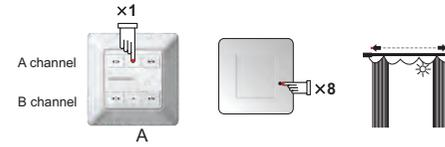
1) Short press the stop button of A channel of emitter A once, and then the learning button 8 times, the motor will vibrate and the power light off.
