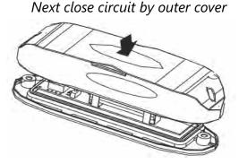
Place the cover over the mounting plate and click into place with a small sideways push.
