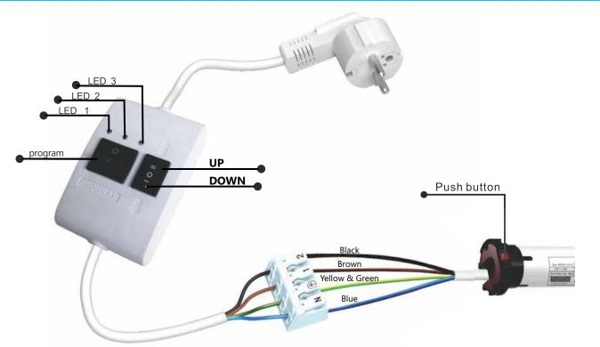
**Notes:** When UP/Down/Program button is pressed, light LED1 is on. When Program button is pressed for 2s, light LED2 is on. When Program button is pressed for 10s, light LED2 is off and LED3 is on.
