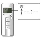
Press K3 until above display appears, which means the point has closed. Press K3 again to retrieve this point.
