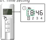
Press K1 button to enter hour setting page, now the hour figure will shine. Press UP/DOWN button to adjust the hour figure.
