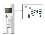
Once the hour setting is finished, press K1 again to adjust minute, the minute figure will shine. Pres UP/DOWN button to adjust the figure.
